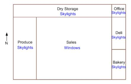
Figure 3-18 Potential Daylight Sources for Each Zone
