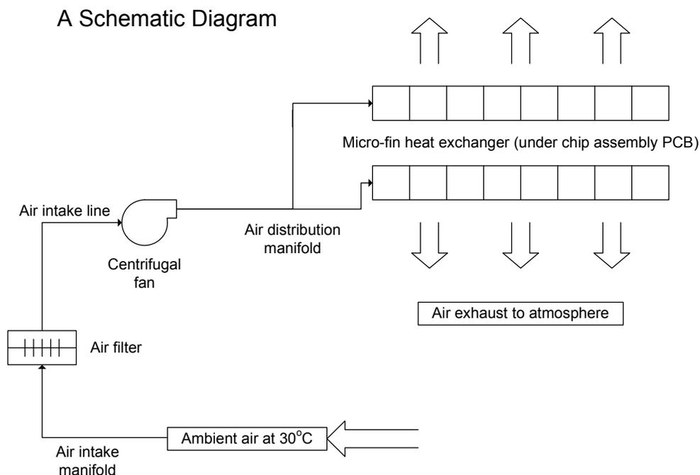
Figure 10. Schematic diagram for cooling power electronics with air
