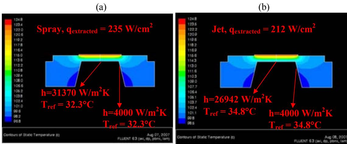
Figure 9. (a) Performance of an HFE 7100 spray, (b) Performance of an HFE 7100 jet
