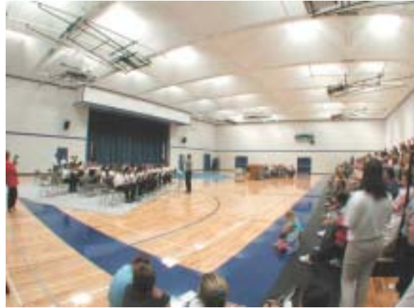
A multi-purpose room should have at least two independent lighting systems for flexibility of use. NREL/PIX 11436
