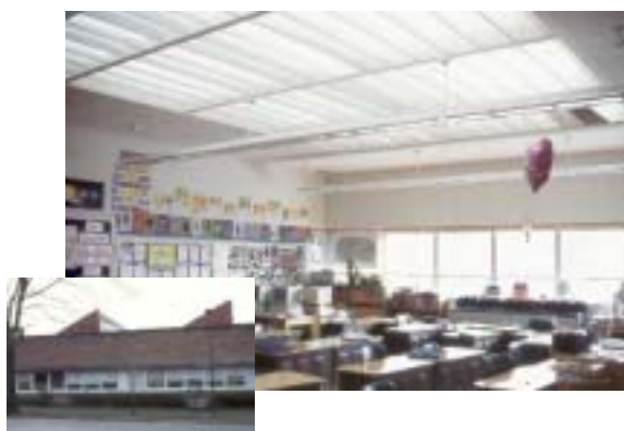
Guideline DL5: Central Toplighting from a sawtooth monitor with sun baffles is combined with DL1: View Windows to provide balanced illumination in a classroom. NREL/PIX 11406
