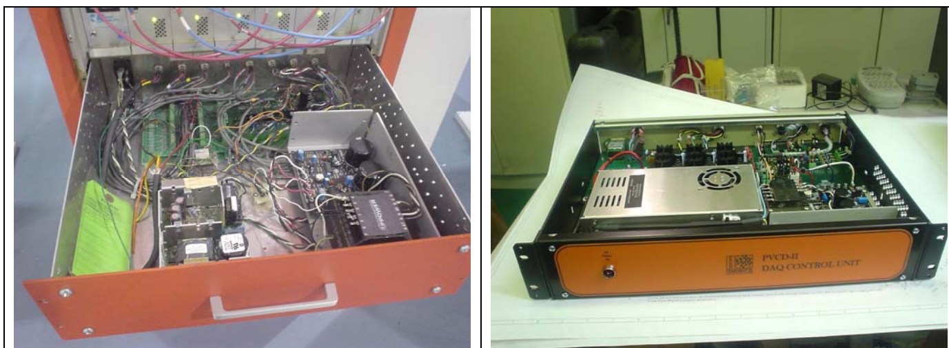
Fig. 3.23. PVCD electronics chassis – Left: development chassis used in the first 25 MW production plant; Right: new professionally-packaged PVCD electronics chassis developed for the 2 nd 25 MW facility.
