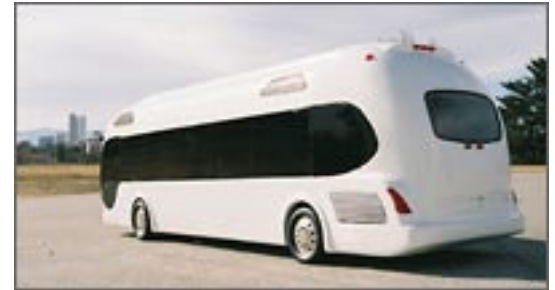
This three-foot model represents the full-size, composite-bodied, hybrid fuel cell bus MES designed for the demonstration project.
