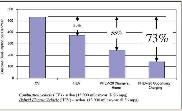
Figure 2. Comparative Fuel Consumption for PHEVs
