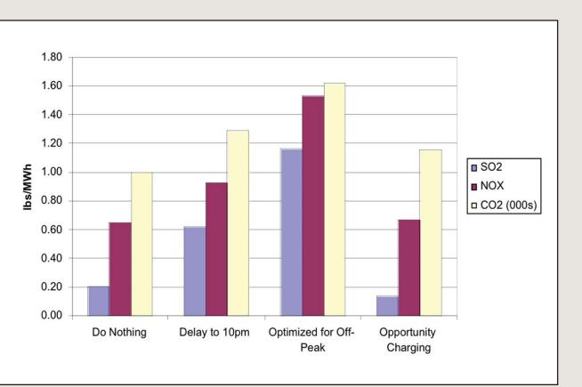
Figure 5. Upstream Emission Rates Impact of PHEVs (50k Vehicles)
