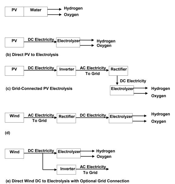
Figure 6. PV and wind electrolysis configurations
