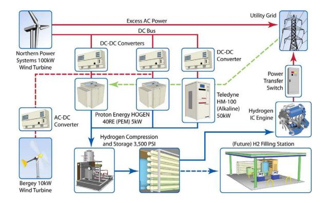
Figure 16. Xcel-NREL Wind2H2 project diagram
