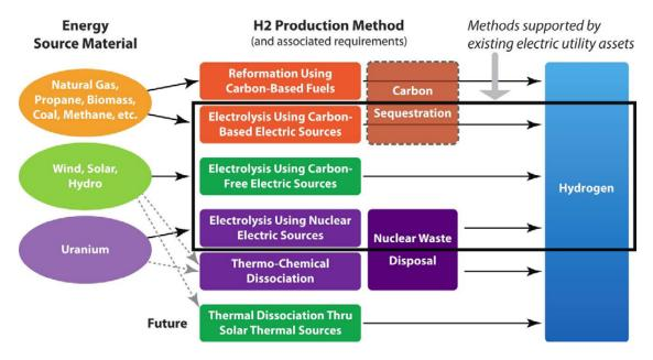
Figure 3. Hydrogen production pathway
