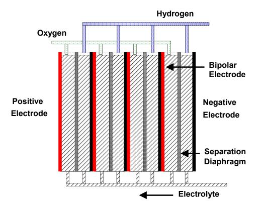
Figure 5. Picture of the bipolar (filter-press) design
