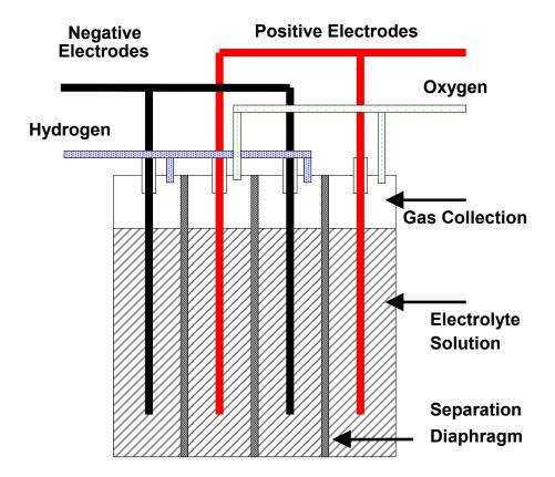
Figure 4. Picture of the unipolar (tank) design
