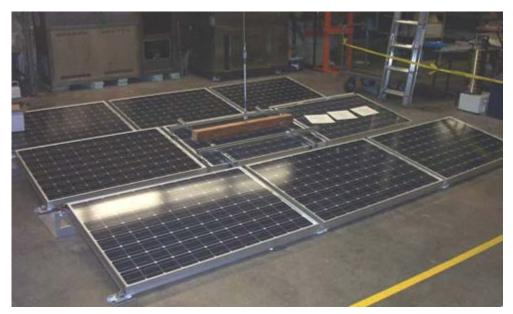
Figure 40: Uplift test on an array of RFT10 tiles. A vertical force is applied to the center tile.
