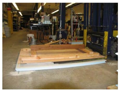
Figure 30: Tensile test of PowerGuard tile made with continuous process
