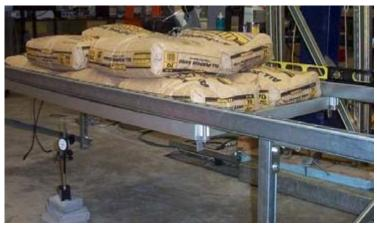
Figure 41: Loading test on a PV module supported with RFT10 mounting clips.
