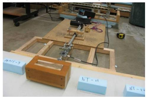
Figure 25: Shear test on XPS spacer bonded to mortar.
