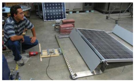
Figure 38: Lateral load test on RFT10 assembly. A compressive load is applied to the north side of the tile.
