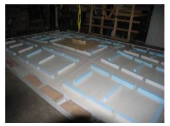
Figure 29: Tile uplift test.
