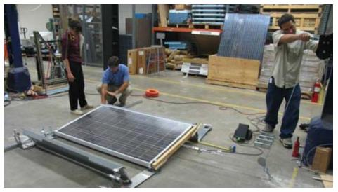
Figure 39: Lateral load test on an RFT10 assembly. A tensile load is applied to the east side of the assembly.
