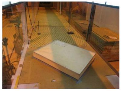
Figure 37: Wind tunnel model for an RFT10 array installed on the edge of a building.
