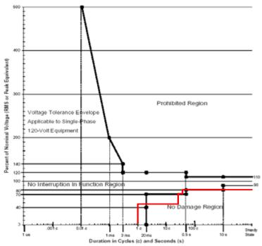
Figure 12. The ITIC/CBEMA and SEMIF47 curve (red)
