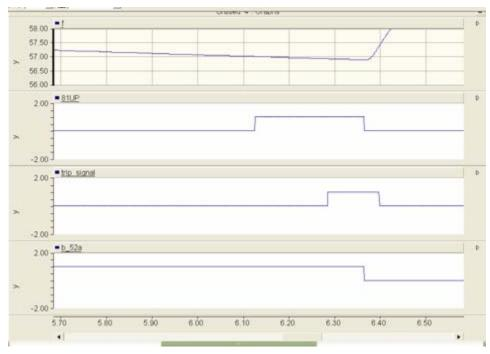
Figure 8. 57 Hz underfrequency
