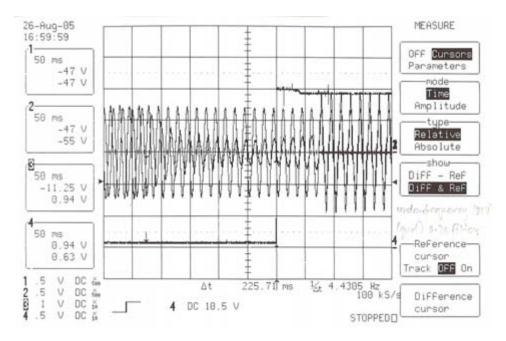
Figure 27. Response of the system to an underfrequency event
