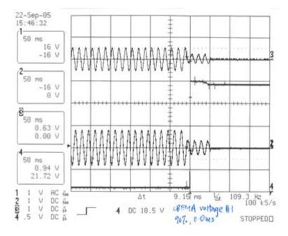
Figure 30. Response to CBEMA (CBEMA voltage #1)
