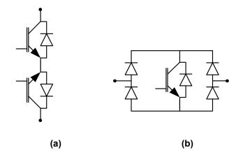
Figure 15. Topology options for the bidirectional switch
