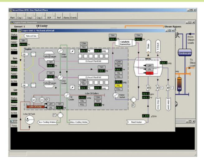
Cogen Mechanical Detail - local HMI access
