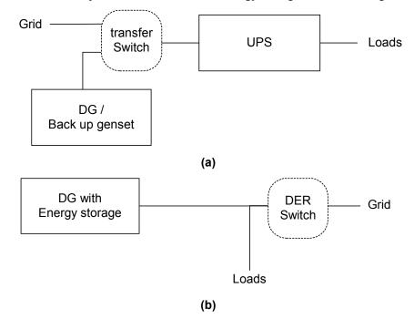
Figure 6. Power system configurations to feed loads with high power quality requirements: (a) Traditional UPS configuration (b) Configuration based on DER Switch.
