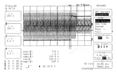
Figure 26. Response of the system to overvoltage event
