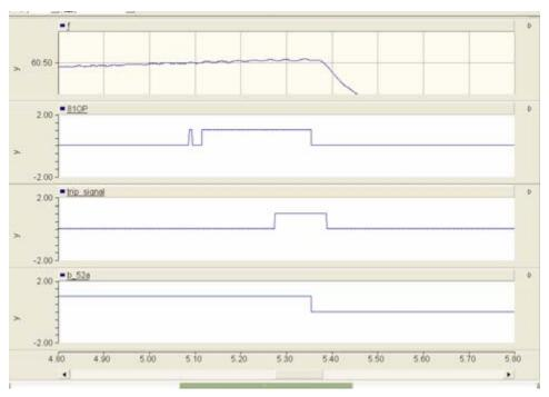
Figure 7. 60.5 Hz overfrequency
