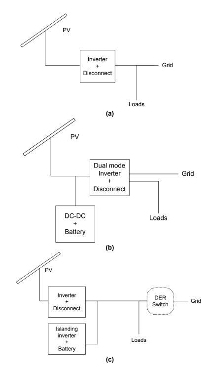
Figure 2. Architecture options for PV installations: (a) grid-connected PV system, (b) PV system with dual mode inverter, (c) grid-connected PV inverter upgraded for intentional islanding capability.
