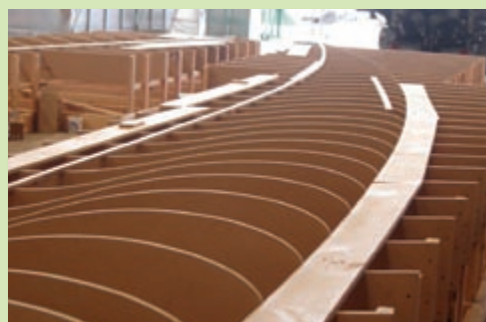
The initial mold fabrication for Knight and Carver's sweep twist blade.
