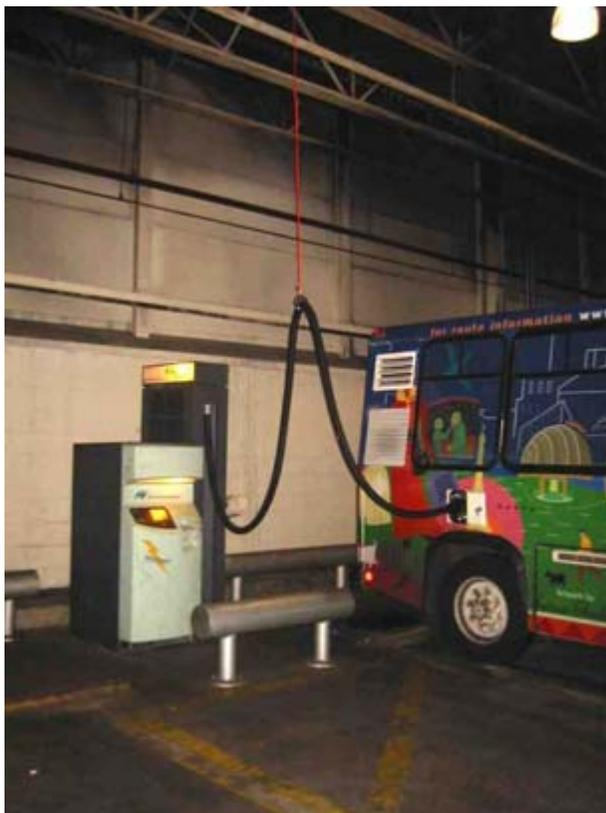
**Figure 15. IndyGo Ebus at Charging Station (Source: NREL)**
