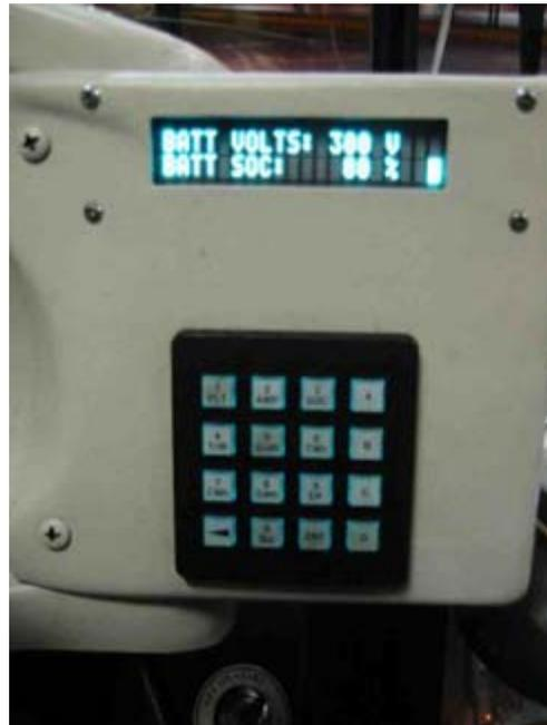
**Figure 17. Battery Charger Display** (Source: NREL)
