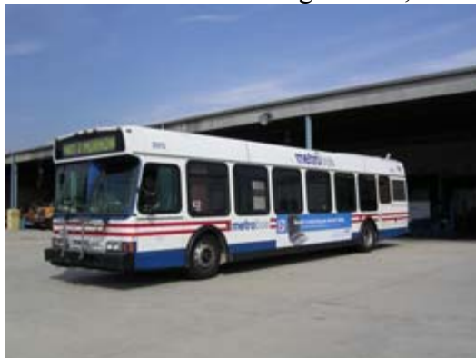
Figure 2: MY 2000 Orion Model 06.501 Bus with MY 2000 DDC Series 50 Diesel Engine
