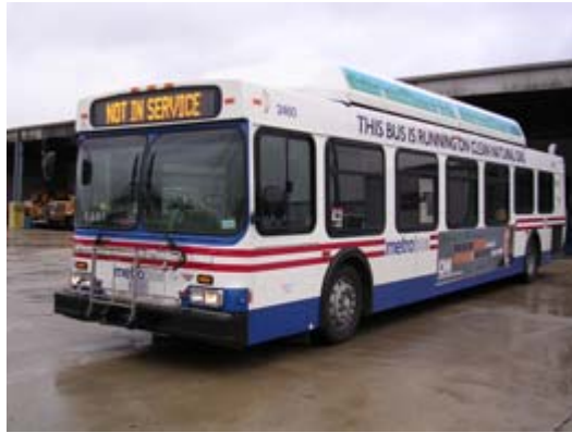
Figure 5: MY 2001 New Flyer C40LF Bus with MY 2004 John Deere 6081H CNG Engine
