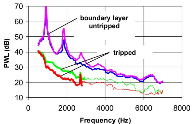
**Figure 4.** Airfoil noise spectra from wind tunnel tests exhibit pure tones (seen as spikes in the upper two curves) resulting from laminar boundary layer vortex shedding. Tripping the boundary layer eliminates pure tones (spikes disappear) and reduces sound levels across the frequency range (broadband noise).
