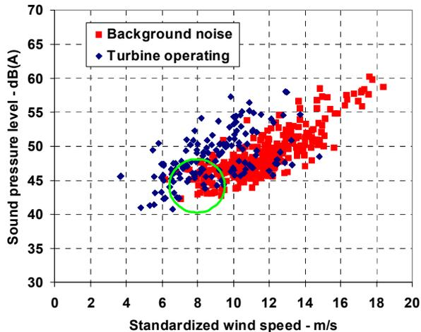
**Figure 2.** The chart compares the noise signature (sound pressure level) of an operating Bergey XL.1 turbine to background noise. Measurements were taken a distance of approximately 10.25 m downwind of the rotor.
