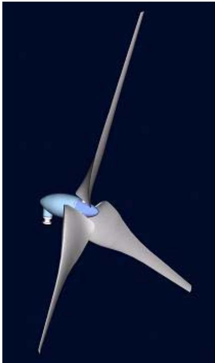
**Figure 1.** Early depiction of the *Storm* turbine illustrating visual simplicity and appealing shapes. The baseline blade was optimized for aerodynamic performance. Large chord and twist near the blade root yield good low wind performance.
