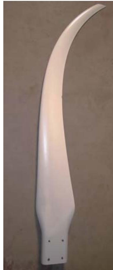
**Figure 11.** Southwest believes swept blades have promise for reducing aeroacoustic noise. These prototype blades will be tested at the NWTC.
