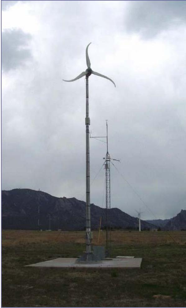
**Figure 15.** *Storm* prototype turbine is being tested at NREL's National Wind Technology Center.
