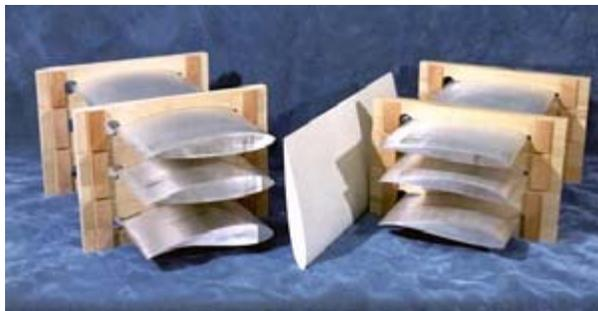
**Figure 3.** Design choices relied heavily on wind tunnel aerodynamic and aeroacoustic data obtained from NREL-contracted tests. References 4-6 provide detailed information on the S822, S834, SG 6043, SH 3055, FX63-137, SD2030, and benchmark NACA 0012 airfoils that were tested.
