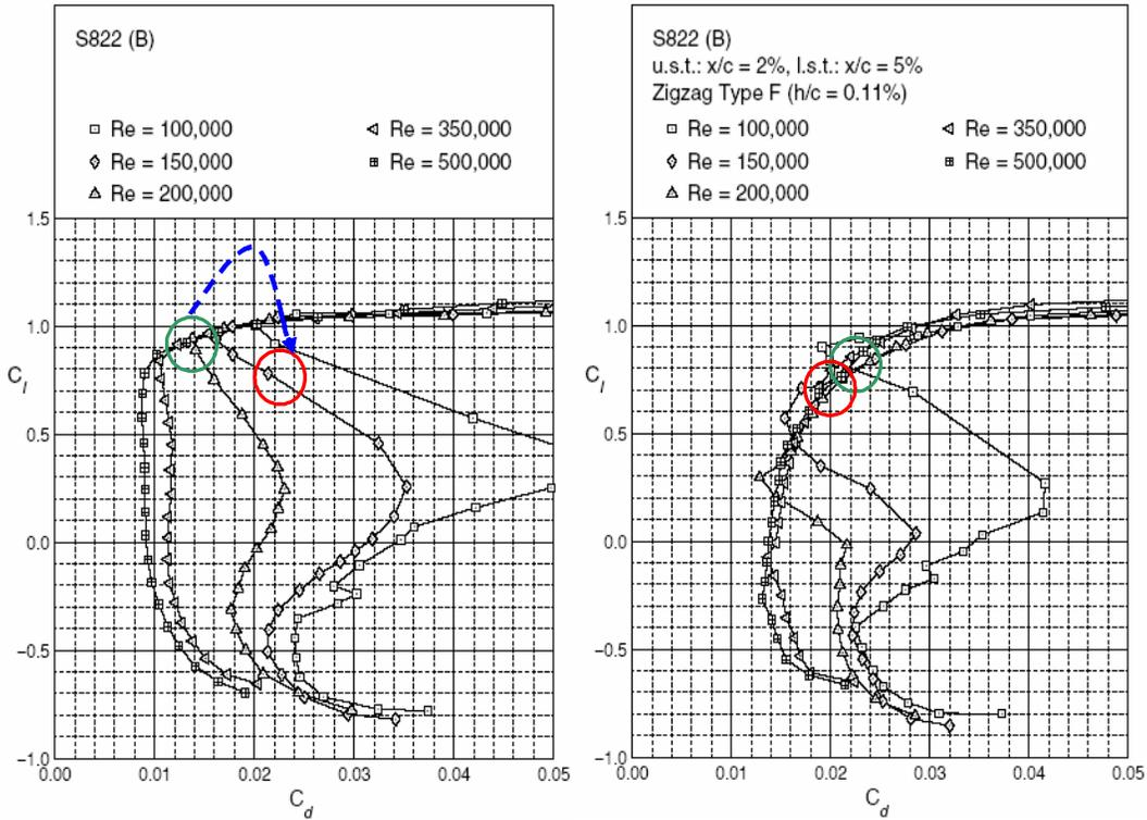
**Figure 7.** Wind tunnel data indicate that airfoil aerodynamic behavior is very sensitive to  $Re$  in the range tested. The data collapse somewhat and are less sensitive to  $Re$  when the boundary layer is tripped (right graph) than when the boundary layer is untripped (left graph).
