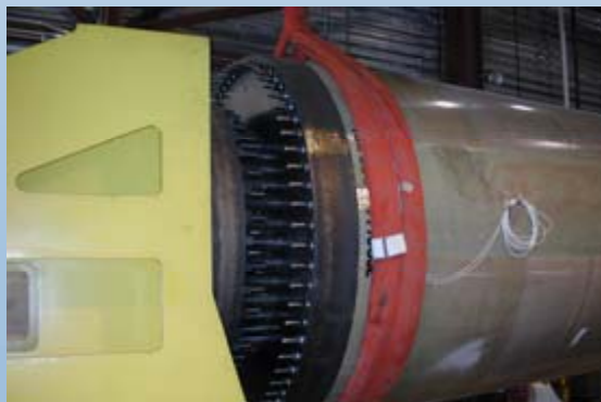
Single-axis Flap Fatigue Test Using B-REX Test System.
