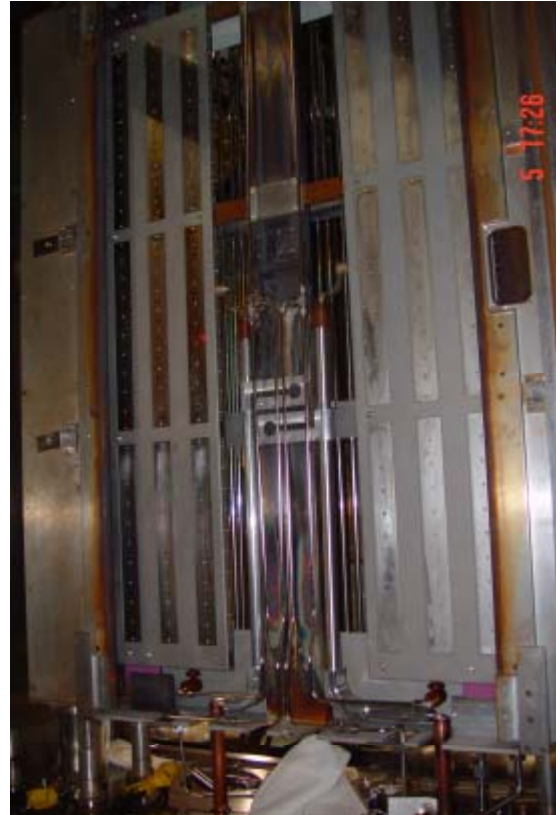
Fig. 3.1. Photograph of the test chamber showing the newly-installed p-type cathodes and gas lines.
