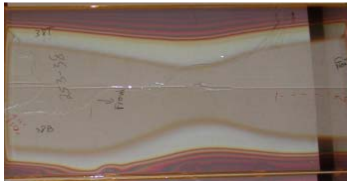
Figure 16: Effect of Glass Spacer between Electrode and Glass Substrate
