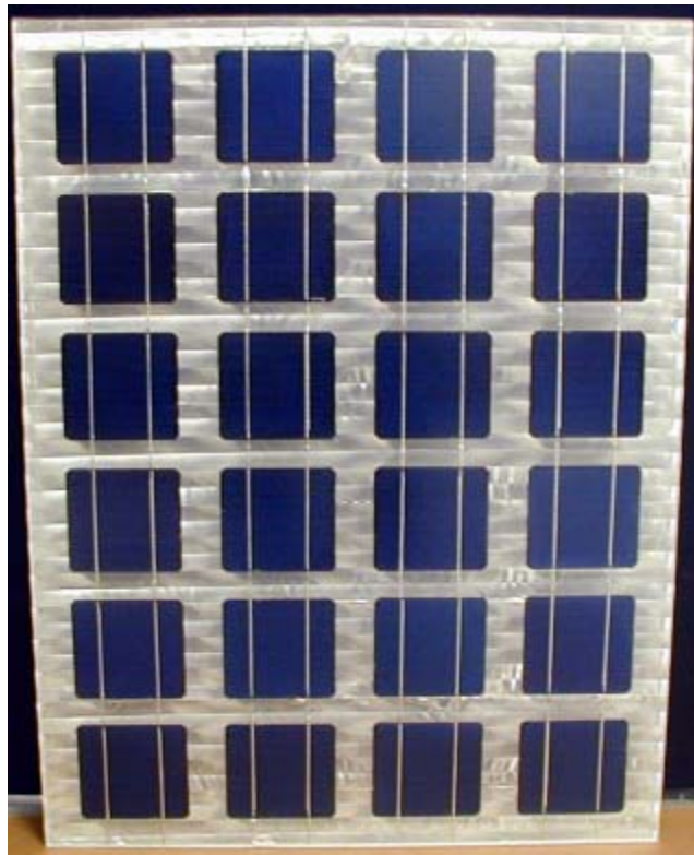
Figure 3. Reflector module incorporating design using 10 cm x 10 cm area cells.
