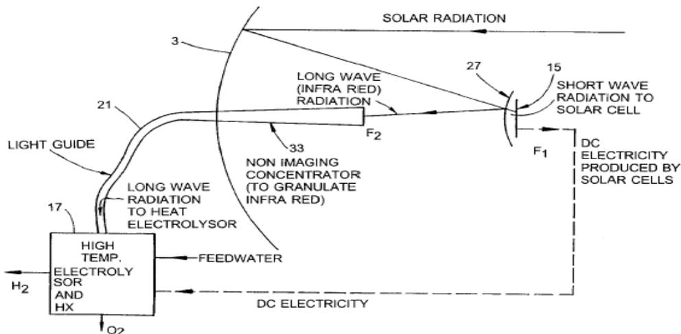
Figure 1. CPV/High Temperature Electrolyzer [1]
