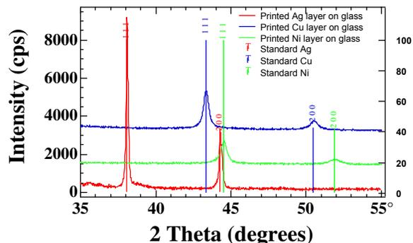
Fig 2. X-ray diffraction patterns of the spray-printed organometallic precursor inks.
