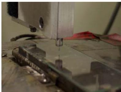
Fig 1. Inkjet printhead positioned over a glass substrate.
