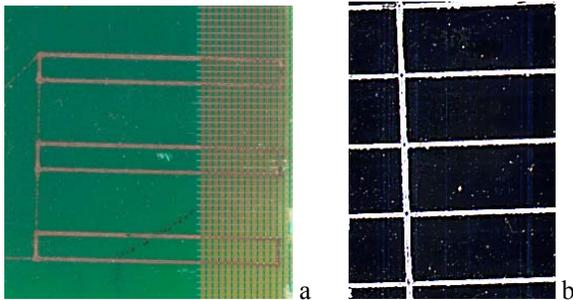
Fig. 3. 300- $\mu\text{m}$ -wide, 5- $\mu\text{m}$ -thick Cu lines printed on PCB in  $\text{N}_2$  at 200  $^{\circ}\text{C}$  (a); 250- $\mu\text{m}$ -wide, 10- $\mu\text{m}$ -thick Ag grids inkjet-printed on a Si solar cell in air at 200  $^{\circ}\text{C}$  (b).
