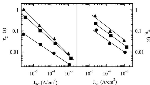
Fig. 1. Characteristic times for collection ( $t_c$  – left panel) and recombination ( $t_R$  – right panel) for dye-sensitized solar cells with nondoped (circles) and doped (squares and triangles)  $TiO_2$  films. The triangles represent the most heavily doped film. The lines are power-law fits to the data.
