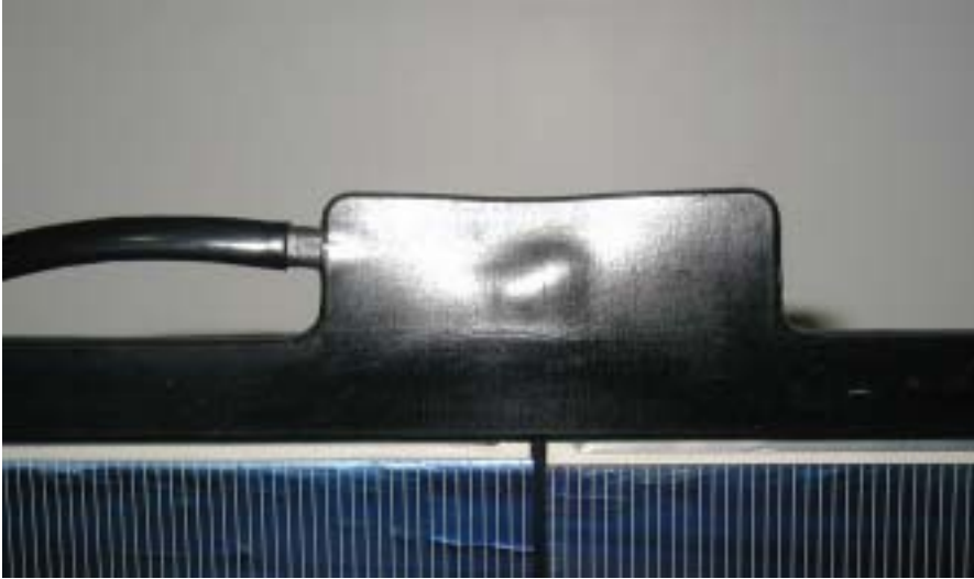
Figure 20 – Top front of a monolithic module showing the region where the leads emerge from the module.
