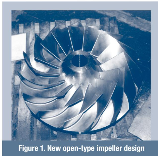
Figure 1. New open-type impeller design
