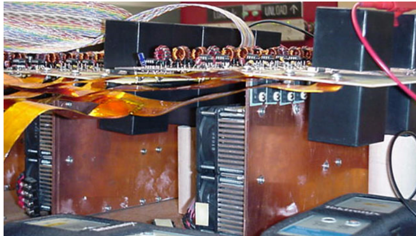
Figure 4-4. Side view of two printed circuit boards. Heat sinks and fans can be seen, mounted on the copper heat spreaders. The black rectangular objects are the DC polypropylene capacitors.
