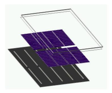
Figure 7 – Showing the layout of a monolithic module. The backskin material with the printed bars of conductive adhesive is at the bottom, the wrap-around cells are shown in blue, a transparent encapsulant layer and finally a superstrate of glass are shown.
