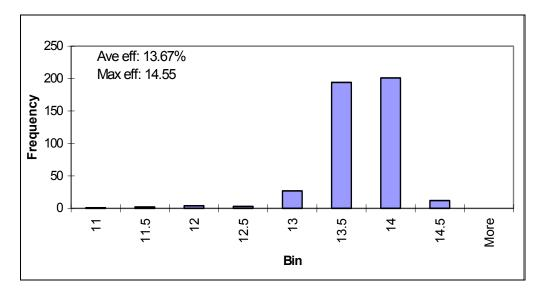
Figure 5 - Efficiency Histogram of Gemini cells
