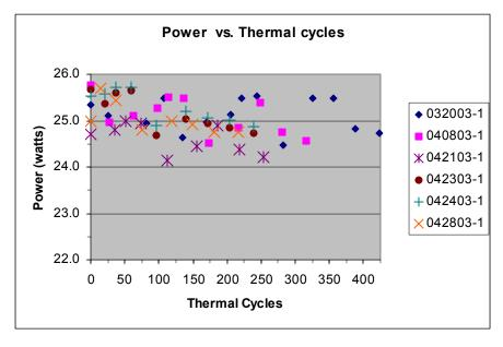
Figure 9 – Thermal cycling data for 25 W size monolithic modules.
