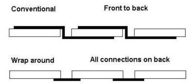
Figure 6 - Showing how a module made with wrap-around cells would differ in interconnection from a module made in the conventional way.
