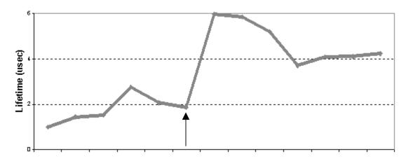
Figure 4 - Starting lifetime before and after improved graphite purification. The arrow indicates when the enhanced graphite purification was introduced.
