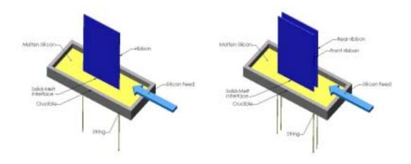
Figure 1a – Single ribbon growth in the String Ribbon process.
