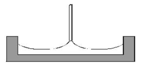
Figure 2 – Illustrating a meniscus shape for a single ribbon in a crucible. Shown is a cross section through a crucible where the ribbon is seen end on.
