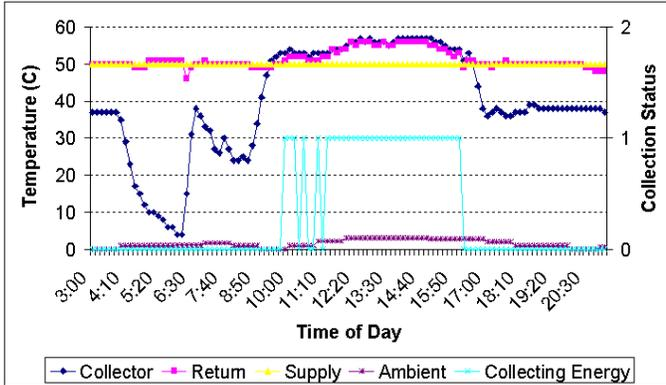
**Figure 4. Collector temperature, recirculation loop supply temperature, return temperature, ambient temperature, and energy collection status (1 = collecting energy) throughout a selected day (January 10, 2004), illustrating the features of system performance**
