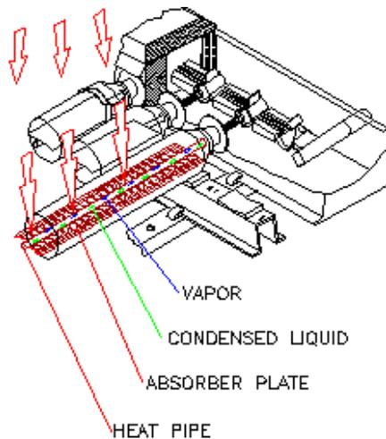
**Figure 3. Components of an evacuated-tube heat-pipe solar collector**
