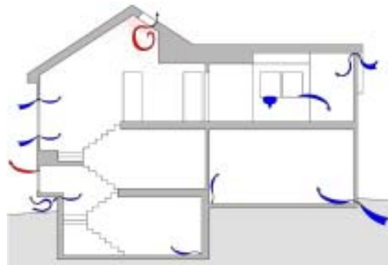
Fig. 28: Gaps in the home should be sealed throughout the rehab process to prevent air leakage and infiltration.
