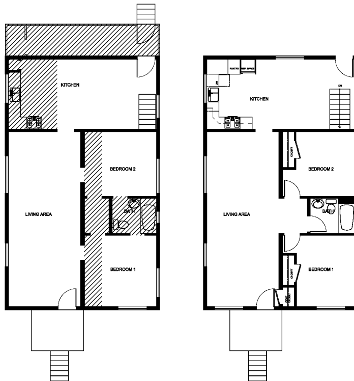
Fig. 3: A better layout is created (right) by revising the original layout (left) and creating a more efficient unit.
