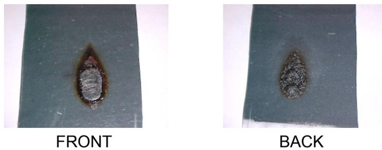
**Figure 10. Flame-Impinged Samples of Halogenated FR Formulation.**
