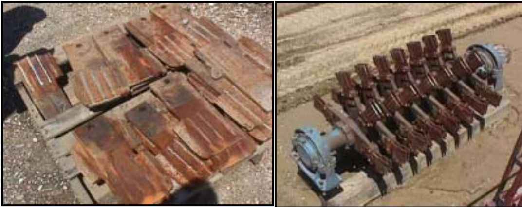
Figure 13 Shredder with Hammers
