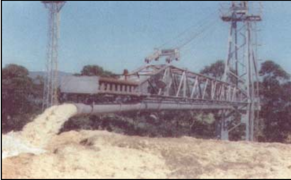
Figure 17 Constructing the Wet Storage Pile: 3% Slurry Discharge
