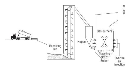
**Figure 2.** Schematic of a typical traveling-grate spreader-stoker.
