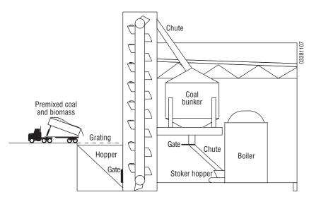
**Figure 8.** A typical stoker boiler conveyor system receiving premixed coal and biomass (Adapted from J. Cobb et al., June 1999).
