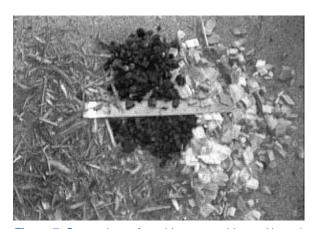
**Figure 7.** Comparison of two biomass residues with coal. Because they are similar in size and flow characteristics, wood chips (right) flow more like coal (center) in stoker boilers. Wood chips can thus be used in existing boilers with minimal modifications to fuel-handling systems. Mulch-like processed wood (left) is more problematic.
