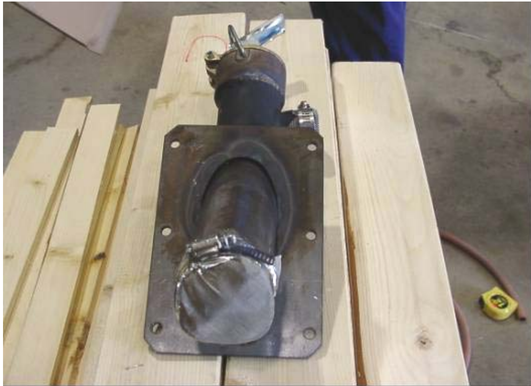
Figure B-14. Fill Neck Removed From Tank No. 4 – Screen Type Flame Arrester Shown (Test 4.2).
