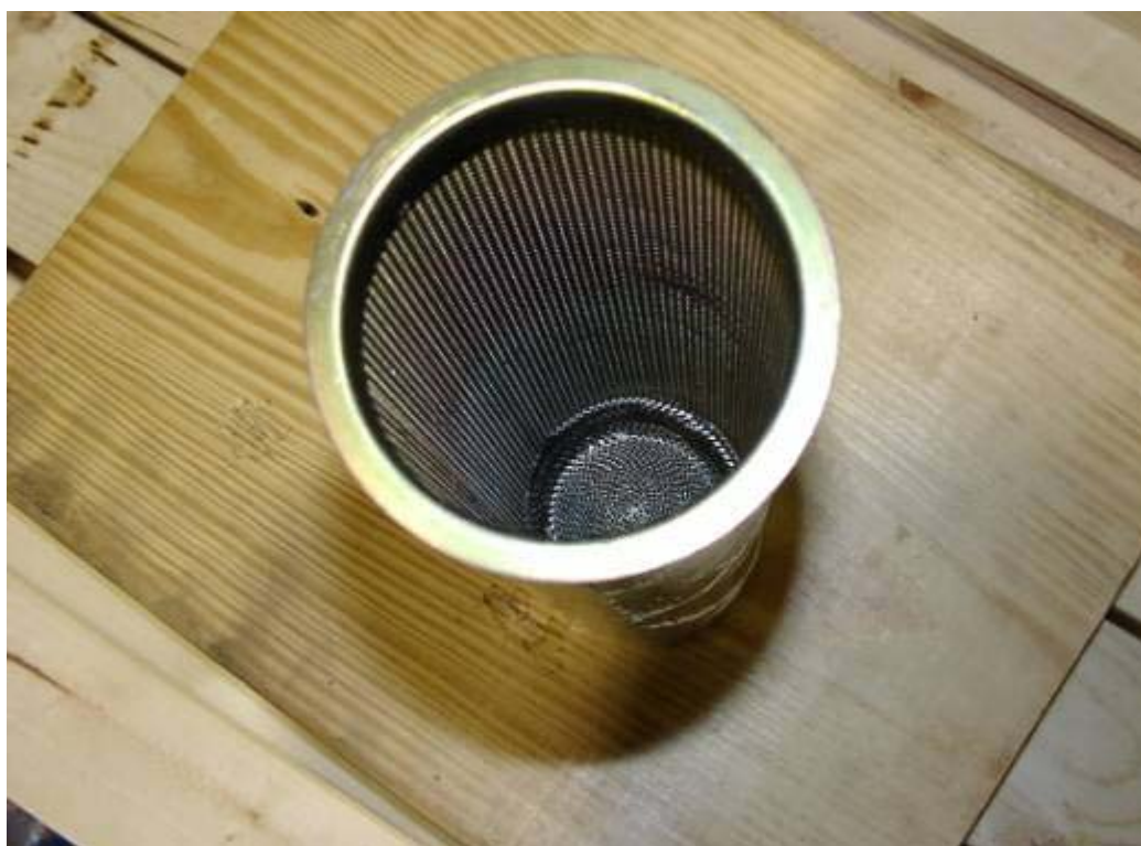
Figure B-8. Brass Fuel Strainer with Stamped Steel Flame Arrester Installed (Test 2.4).
