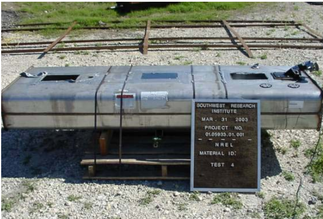
Figure B-15. Tank No. 4 After Typical Failure.
