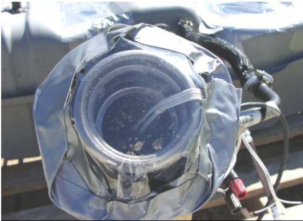
Figure B-10. Tank No. 3 Fill Neck Mouth Shown Prior to Test with Electric Match Installed.
