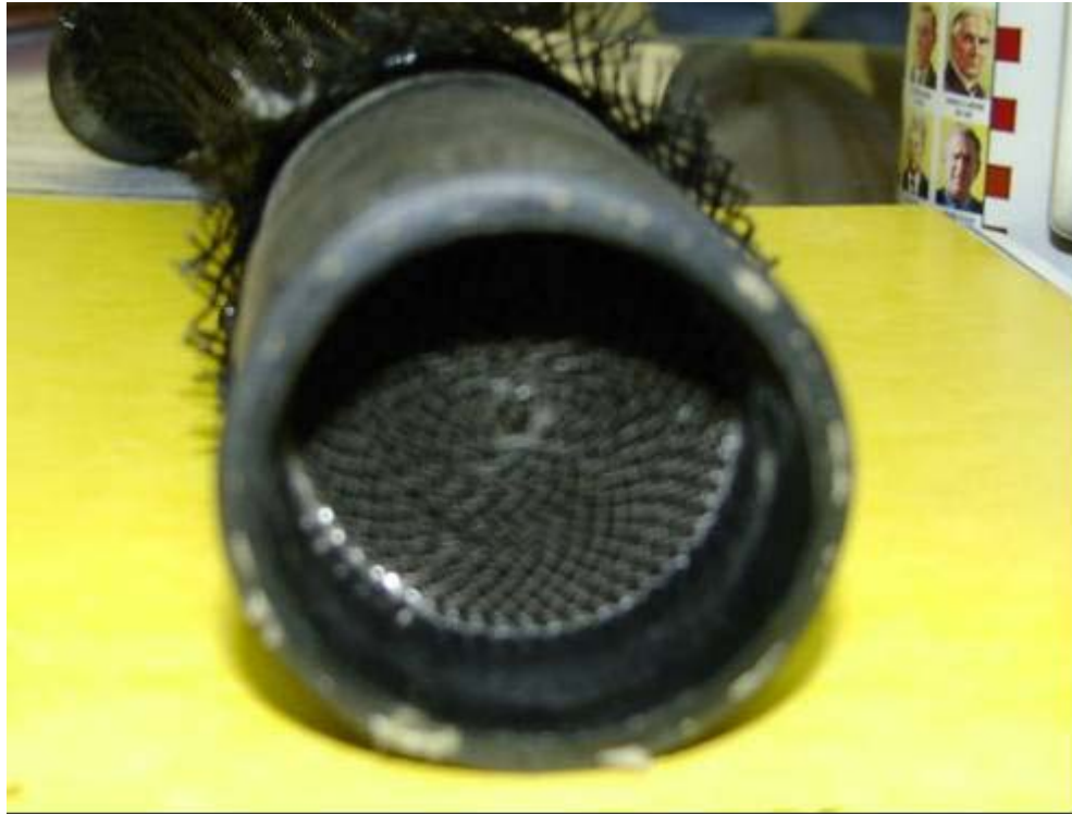
Figure B-11. Tank No. 3 Fill Neck with Stamped Metal Flame Arrester Installed (Test No. 3.2).
