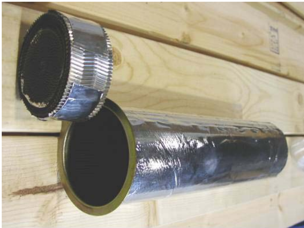
Figure B-7. Brass Fuel Strainer Next to Stamped Steel Flame Arrester (Test 2.4).
