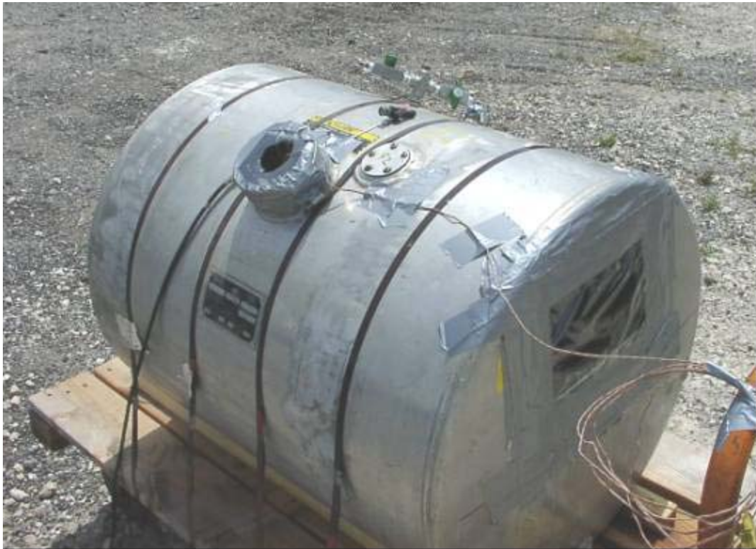
Figure B-4. Tank No. 2 After Typical Flame Arrester Pass.
