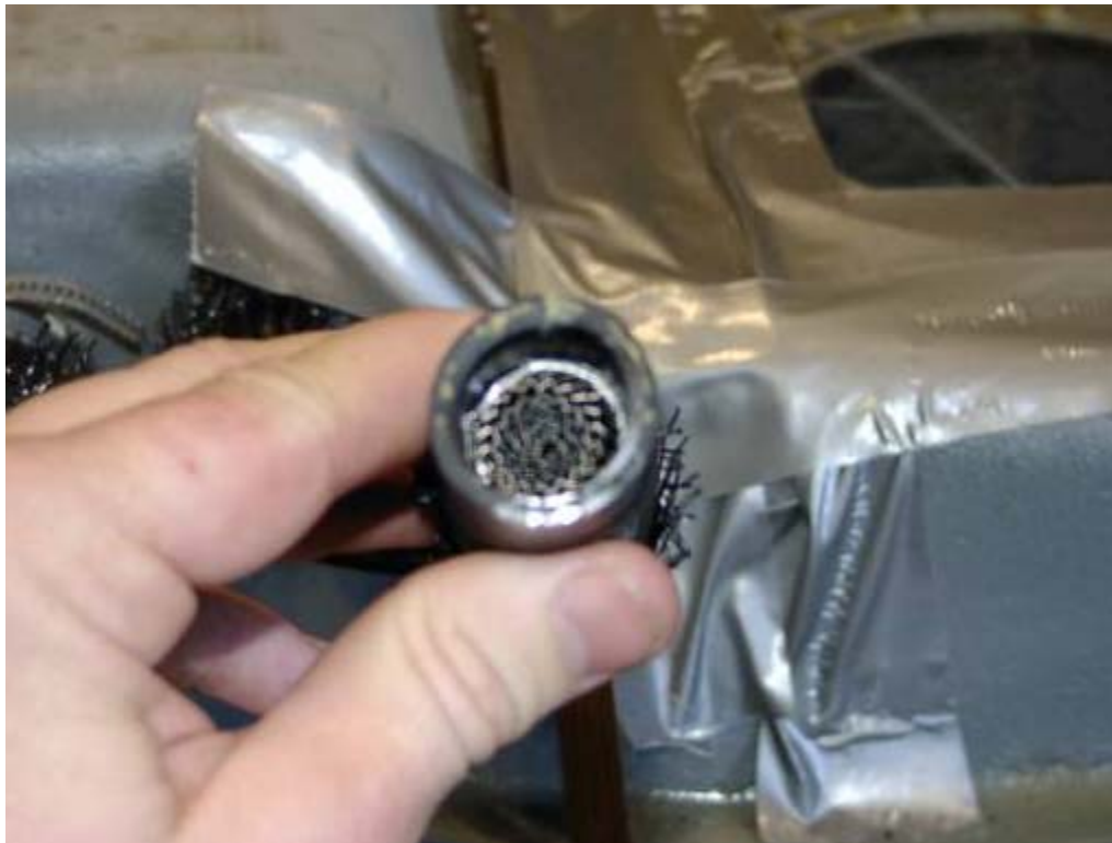
Figure B-12. Tank No. 3 Vent Tube with Stamped Metal Flame Arrester Installed (Test No. 3.2).
