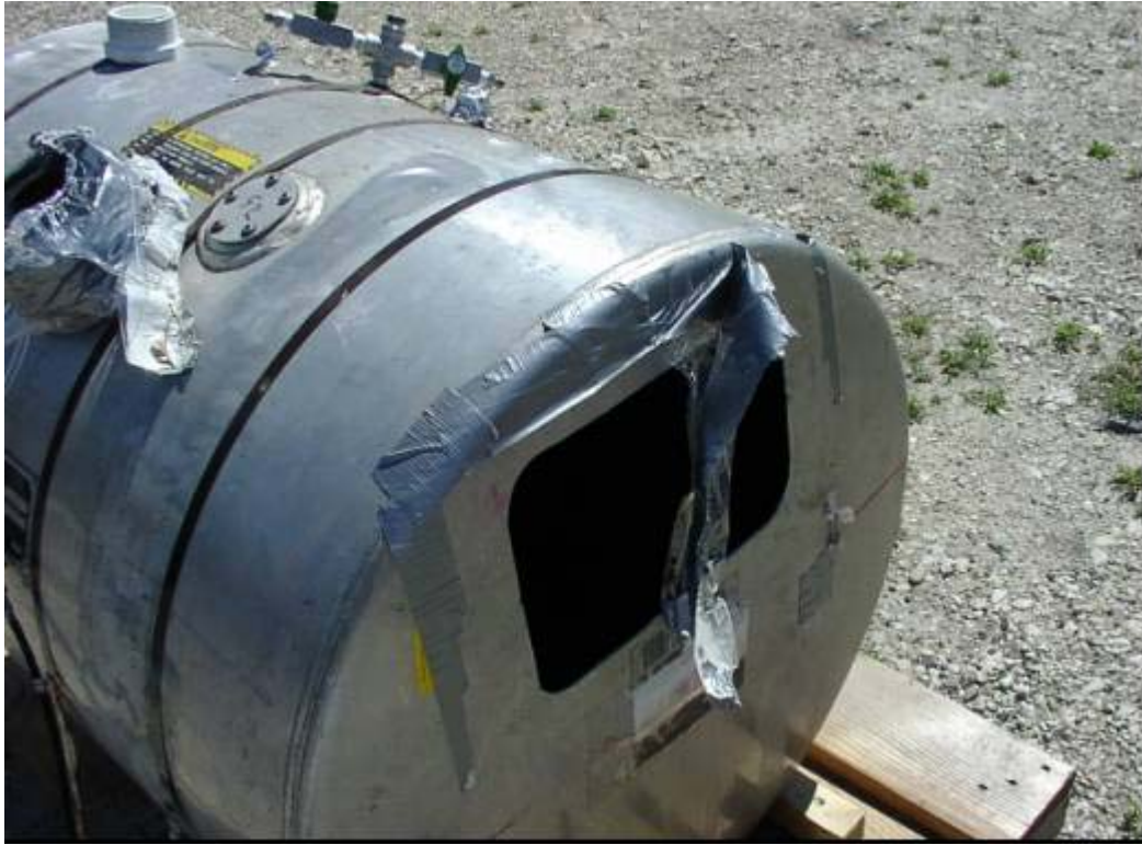
Figure B-3. Tank No. 1 After Typical Flame Arrester Failure.
