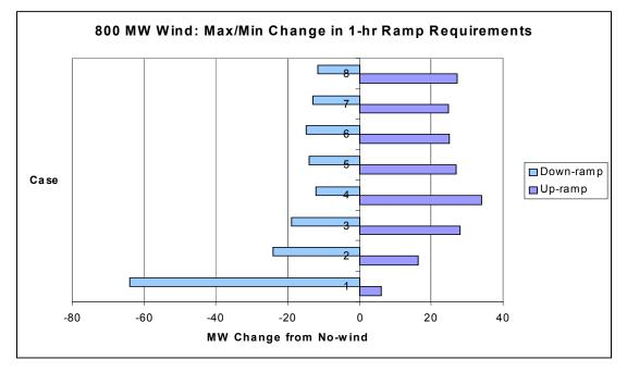
FIGURE 7. MAXIMUM CHANGE IN RAMPING REQUIREMENTS FOR 800 MW OF WIND CAPACITY.
