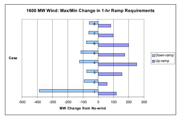
FIGURE 8. MAXIMUM CHANGE IN RAMPING REQUIREMENTS FOR 1600 MW OF WIND CAPACITY.
