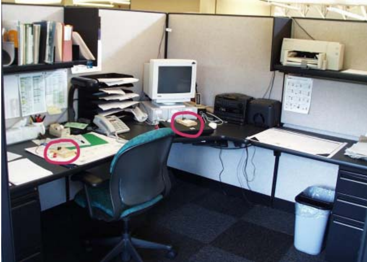
Figure 12. Placement of photometers (shown circled) on the working plane in a typical cubicle
