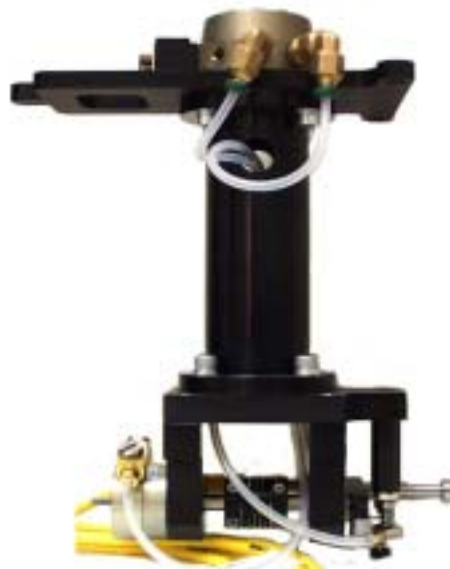
Figure 56 Tab lift end-effector.
