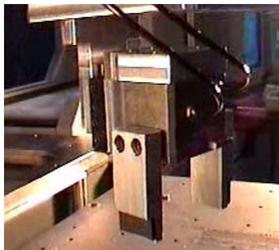
Figure 48 J-box pick-and-place end-effector.
