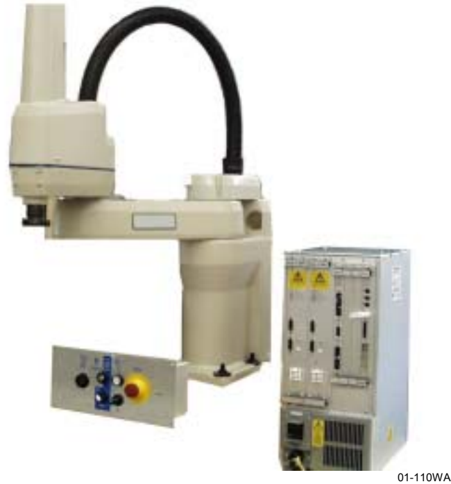
Figure 60 Four-axis SCARA robot for the J-box installation system. The robot controller is shown at right; the controller interface panel is at left.
