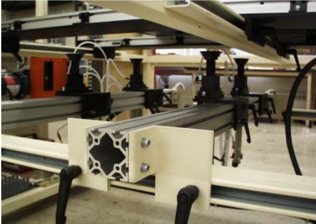
Figure 33 Module vacuum lift, retracted under belt conveyors.
