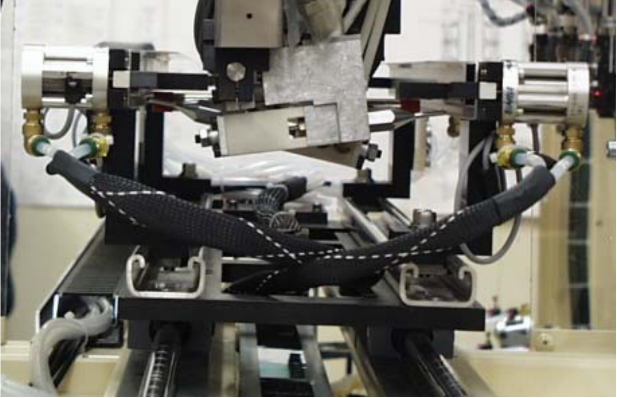
Figure 38 Sealant dispense nozzles over short frame carriage.
