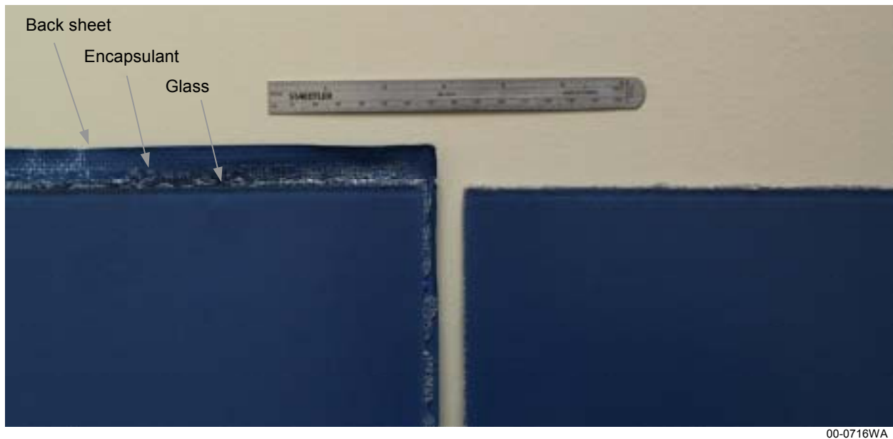
Figure 35 BP Solar laminates before (left) and after (right) trimming with SPI-TRIM 350.
