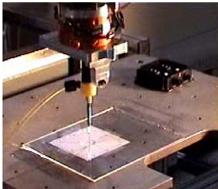
Figure 45 Alcohol dispense end-effector.
