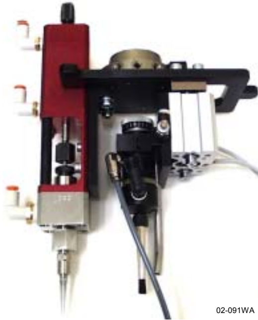
Figure 54 Robot end-effector for cleaning and sealant dispensing.
