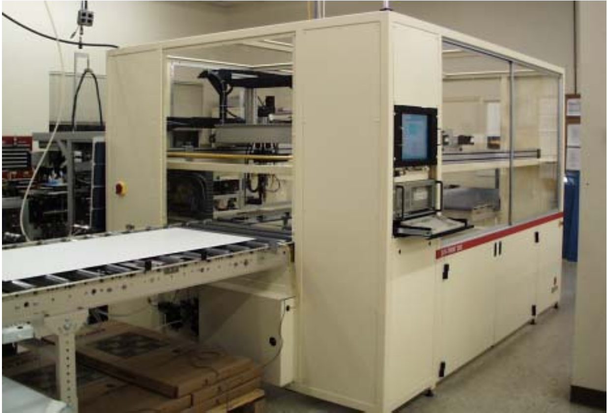
Figure 31 SPI-TRIM 350 automated module edge trimmer, with module laminate at aligner on in-feed conveyor.
