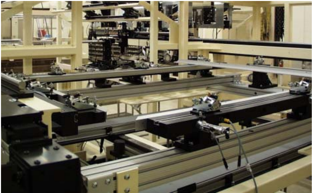
Figure 39 Two-axis frame press.
