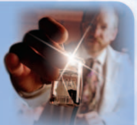
An NREL scientist holds a beaker containing a photolytic device submerged in an alkaline aqueous solution. This configuration produces hydrogen from water with greater than 12% efficiency.
