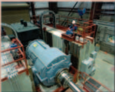
At NREL's Dynamometer Test Facility, a drivetrain for a 750-kW wind turbine undergoes tests to measure loading under realistic conditions and endurance tests to verify design life.
