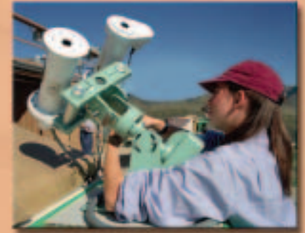
A researcher adjusts an absolute cavity radiometer at NREL’s Solar Radiation Research Laboratory. Absolute cavity radiometers are used to make very accurate measurements of solar irradiance and provide the reference from which other radiometers are calibrated.
