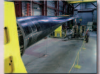
A blade for a 750-kW wind turbine is being fatigue tested at NREL's Industrial User Facility.
