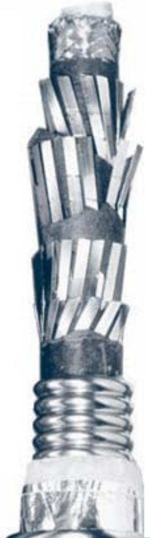
***Cut-away view of an HTS cable. The central tube at the top carries the liquid nitrogen coolant, and the four layers of superconducting tapes in the upper part of the picture conduct the electrical current. Insulation and shielding make up the outer layers of the cable.***
