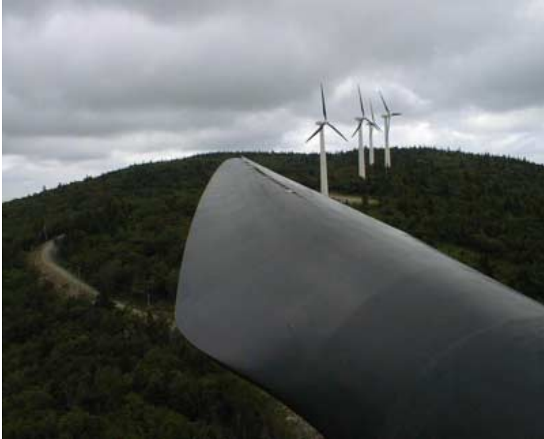
Figure 3. Damaged Zond Z40FS blade at GMP site
