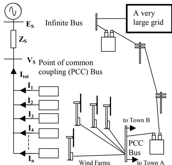
Figure 1. Multiple wind turbines feeding the grid
