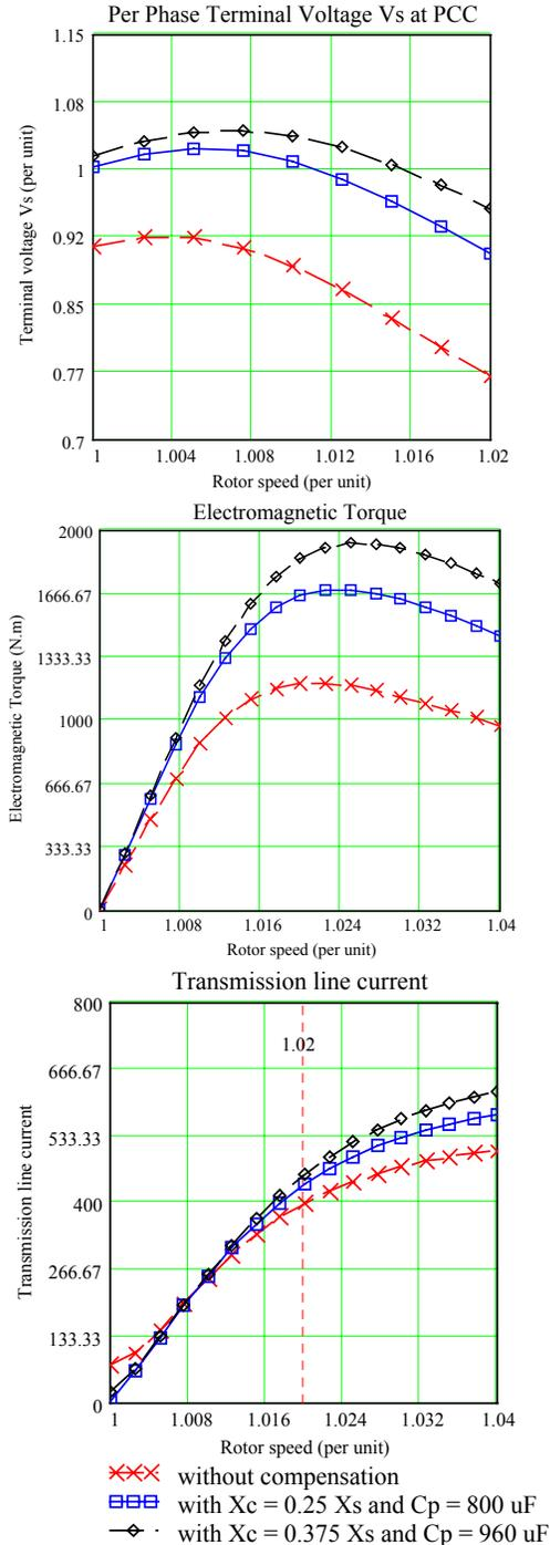
**Figure 16. Parallel and series combination with 300 turbines on-line**
