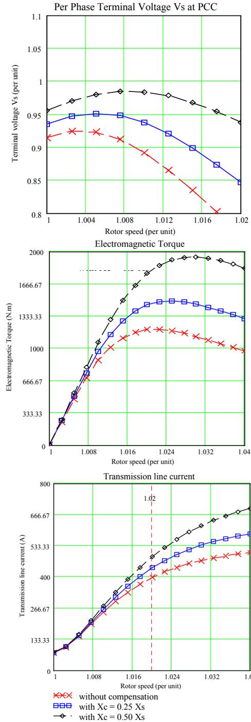
**Figure 13. Series compensated with 300 turbines on-line**
