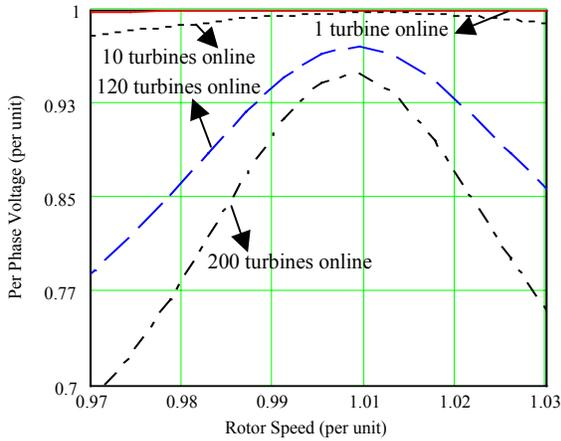
**Figure 5. Per-phase voltage at PCC versus rotor speed**
