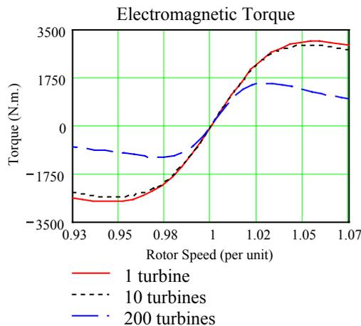
**Figure 6. Torque-speed characteristic of individual induction machine**
