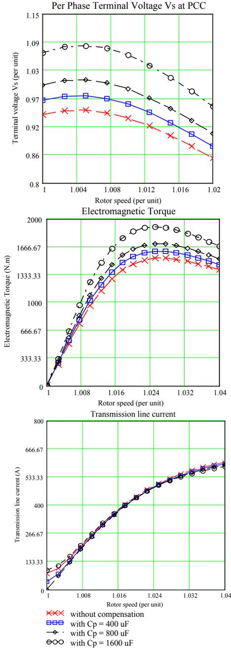
**Figure 10. Parallel compensation with 200 turbines on-line**
