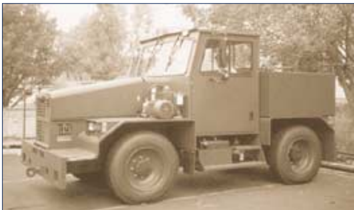
Hybrid-electric tow tractors at Robins mate a Cummins diesel engine with 48 lead-acid batteries and a 100-kilowatt Siemens motor.
