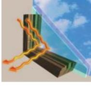
Double-pane windows with low-e coating on the glass reflect heat back into the room during winter months.
