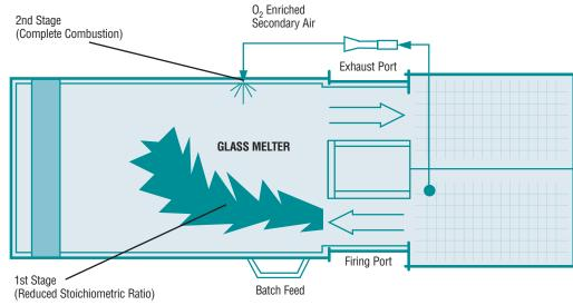
Oxygen-Enriched Air Staging uses a two-stage process to reduce NOx formation. The amount of air entering the furnace is reduced, which not only reduces NOx formation but also yields incomplete combustion. Therefore, oxygen or oxygen-enriched air is injected into the furnace near the exhaust port to complete combustion and heat release.
