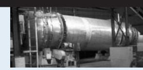
exposing it to a high-temperature, low-O<sub>2</sub> gas, which removes the waste oils without combustion or oxidation. The oil-laden gas is then combusted in an afterburner, apart from the scrap, to destroy the volatile organic compounds (VOCs). The heat released during the oil combustion is then used to drive the decoating process.
