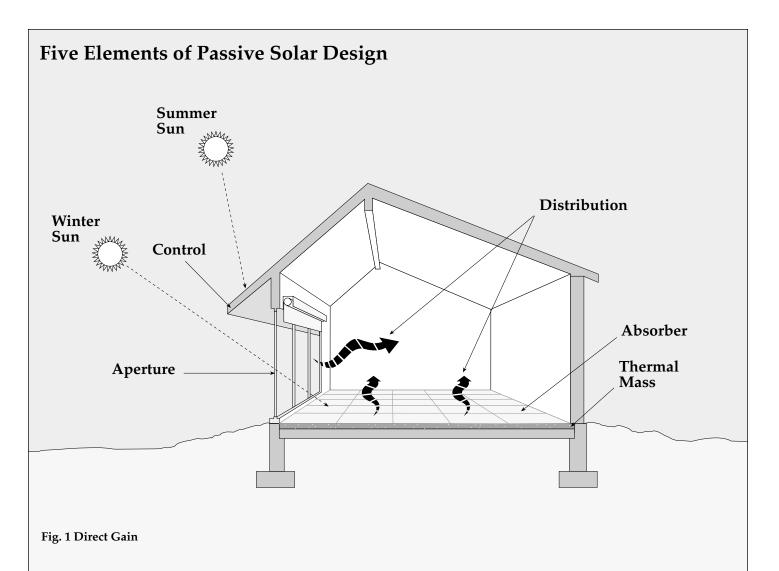
Here are the five elements that constitute a complete passive solar design, using a direct gain design as an example. Each performs a separate function, but all five must work together for the system to be successful.
