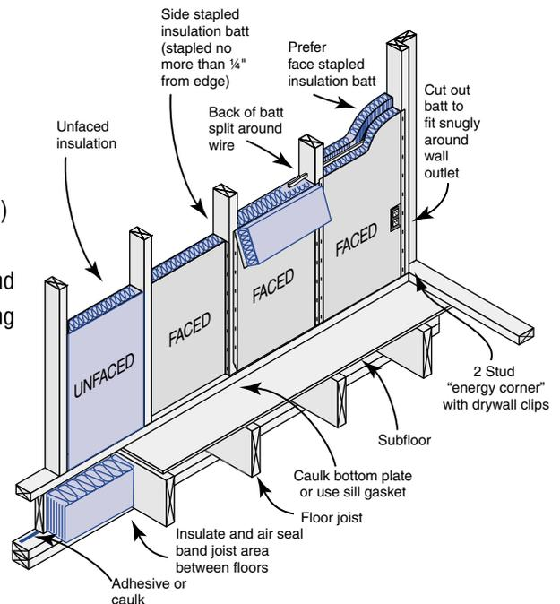
9. Obtain full coverage of batt or blown wall insulation. Cut batt insulation to fit snugly into non-standard stud spaces and to completely fill cavity.
