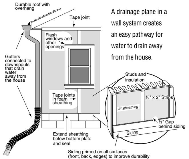
A drainage plane in a wall system creates an easy pathway for water to drain away from the house.
