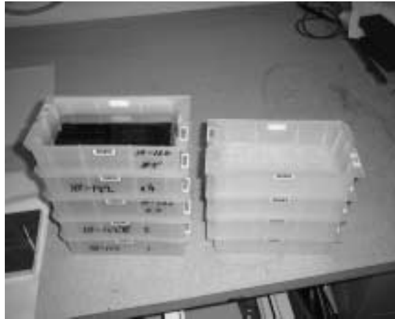
Figure 10 Example of storage and handling boxes. 8 cm wide String Ribbon blanks are in the boxes on the left.
