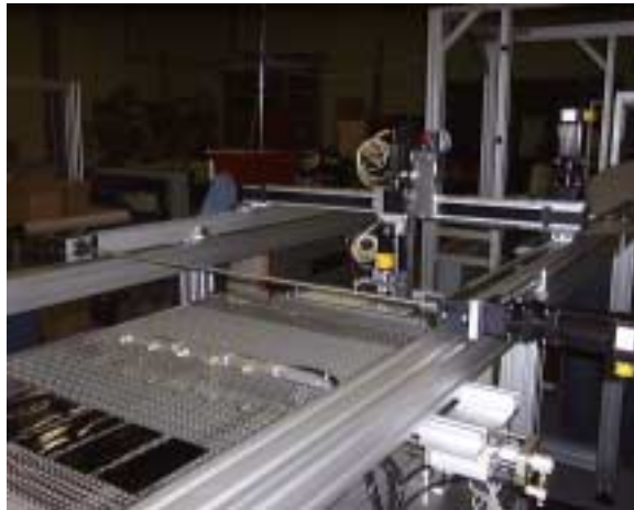
Figure 12 The belt transfer system and generic gantry system.
