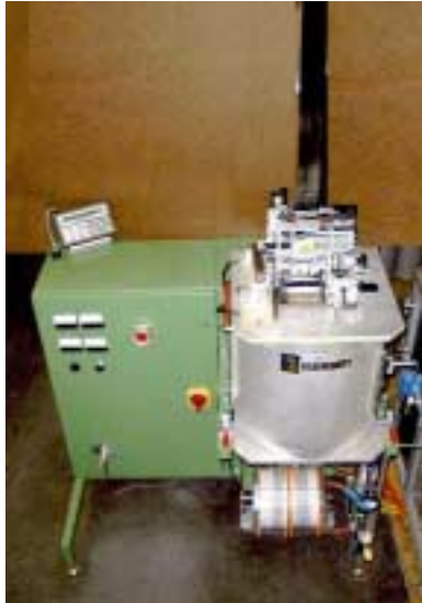
Figure 3 New crystal growth furnace with 5.6 cm wide ribbon growing.
