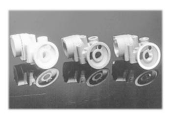
Aluminum transmission housing produced by "lost foam process."
