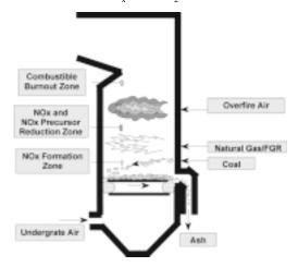
Spreader stoker boiler retrofit with Methane de-NOx technology
