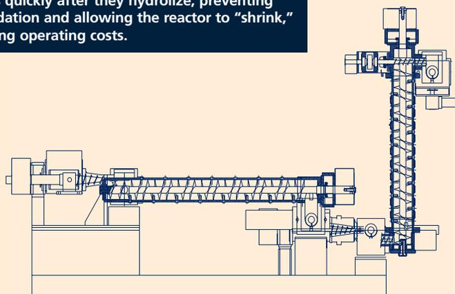
are lifted upward. This not only reduces the amount of hot dilute acid solution needed—a critical consideration in achieving acceptable process economics—but maintains more effective contact between the solid particles and the flowing dilute acid. This is believed to reduce mass transfer reaction resistances, allowing for lower temperatures and lower acid concentrations to achieve the same degree of hydrolysis as in more traditional reactor designs.
