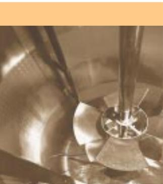
Inside one of four 9000-liter fermentation tanks at the National Renewable Energy Laboratory's Bioethanol Pilot Plant. The facility enables NREL and its industry partners to move advances in producing ethanol and other fuels and chemicals from biomass into the development phase.
