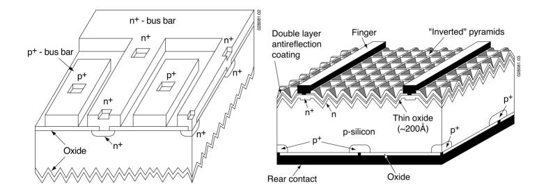
Fig. 2 Rear point contact solar cell
