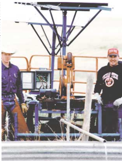
These ranch hands assembled John Buol's PV-powered water pump in just 20 minutes. When Buol moves his herd to another pasture, he takes his pump with him.
