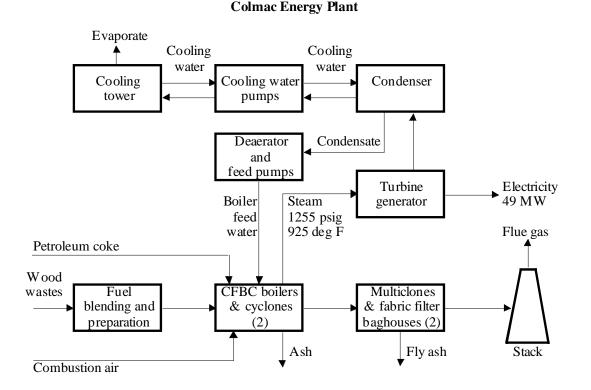
Colmac Energy has made numerous improvements to the boilers to improve operations and reduce maintenance costs. Modifications have been made to the vortex tubes, cyclone separators, grid nozzles, high-efficiency air preheaters, and furnace refractory. Natural gas input, which was required initially for flame stabilization, has been reduced to nearly zero.
