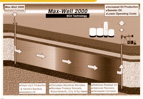
The in situ BCX process suppresses harmful sulfide-producing bacteria and stimulates beneficial bacteria to reduce sulfide production (also known as "sweetening") and mobilize residual oil.
